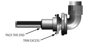
8. Attach the Entry Item (1) by screwing it into place, making sure the compound is not disturbed, and loosely tighten the Nut (3). Leave until the compound has cured.
