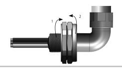
9. When the compound has cured the Entry Item (1) should be removed from the assembly and fully tightened into the apparatus. The Union can then be refitted to it and the Nut (3) fully tightened to complete the installation.
