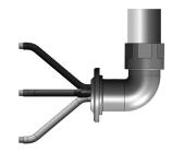
6. Bring the cores together again and pack more compound around them to a length and diameter sufficient to fill the Compound Tube (6) (ensuring compound is packed between each of the cable cores) before ending in a taper.
