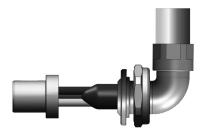
7. Pass the Compound Tube (6) over the conductors until the stepped end is fully located with the Washer (5). Pack more compound into place until the Compound Tube is fully fitted and trim off any excess
